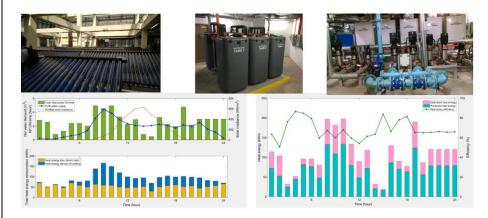
We investigate the energy efficiency of the solar thermal hot water system and identify the issues of the system. Through optimized control, we demonstrate energy saving of 50% is possible. In addition, we also build an AI model for heat pump condition monitoring, which can be used for abnormal detection and predictive maintenance.
